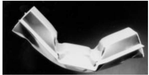
Fig. 5 Bending test, deformed shape of tube filled with 6 pcf density of polyurethane foam
