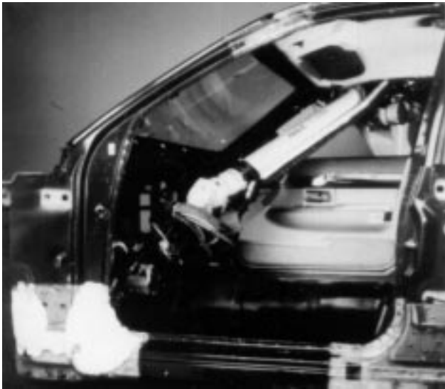
Fig. 2 Current applications are performed manually using a light-weight gun with Foamseal's patented mix chamber. Robotic application is being developed and tested.
