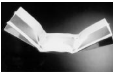
Fig. 4 Bending test, deformed shape of tube filled with 3 pcf density of polyurethane foam
